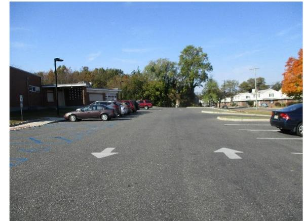
Installing rain gardens adjacent to the building and parking lot can capture, treat, and infiltrate runoff. A preliminary soil assessment suggests that the soils have suitable drainage characteristics for green infrastructure.
